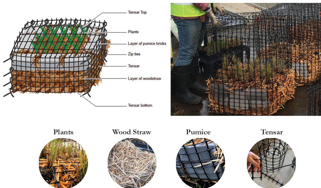
Figure 14. Wetland biofilter 1.0 design. Diagram courtesy of the Green Futures Lab.
