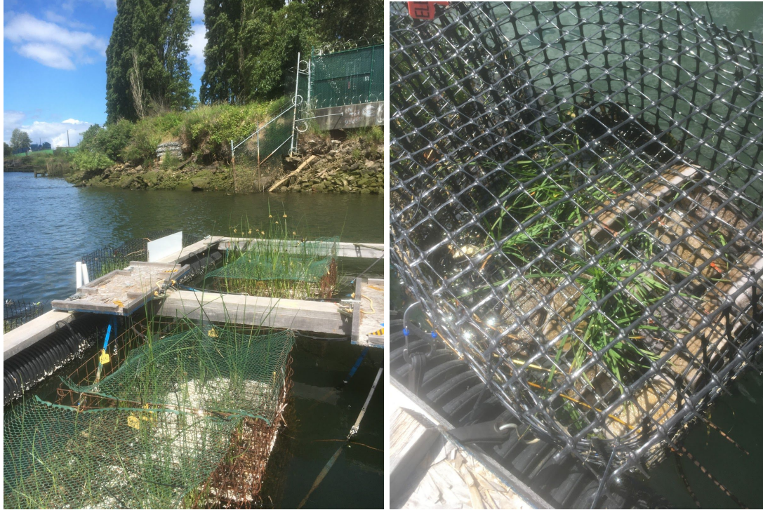
Figure 18. Biofilter damaged by boat wakes at Waste Management. BioBarge (left) sheltered from boat wakes. A biofilter 2.0 (right) which had undergone structural damage from exposure to boat wakes.
